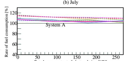
Fig. 18 Analysis results of fuel consumption rate of System B relative to System A. Heat supply to the following buildings: power-generation (A\_0), residence (A\_1, A\_2), warehouse and sewage disposal (A\_3), and administration (A\_4) buildings which are shown in Fig. 1.
