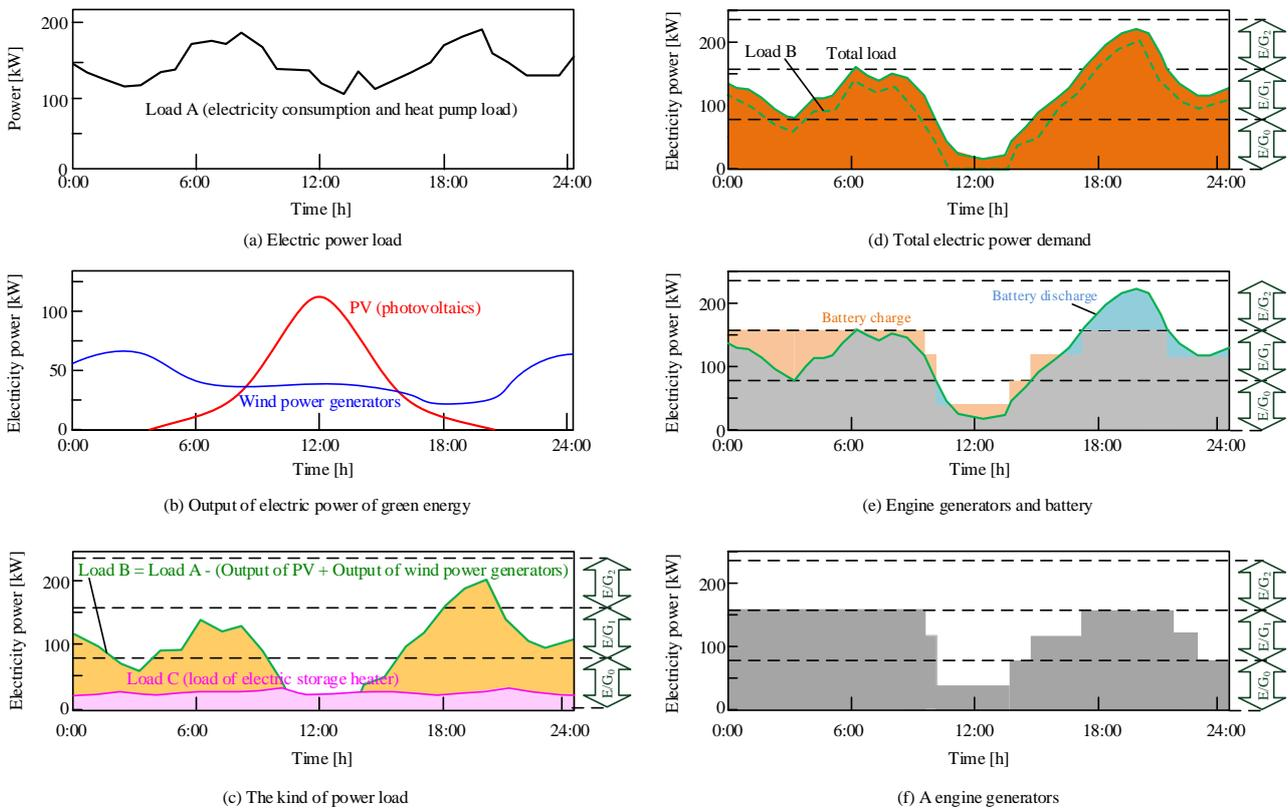
Fig. 3 Proposed operation planning of the SBMG
