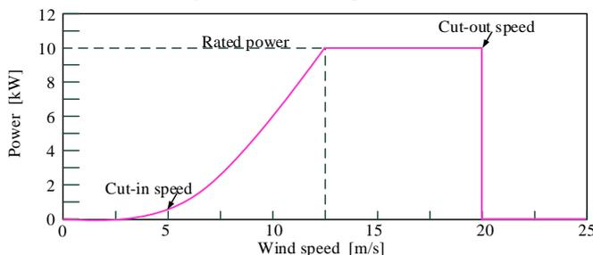
Fig. 7 Power performance of wind power generator
