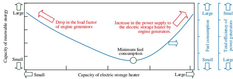
Fig. 19 Capacity optimization of the electric storage heater
