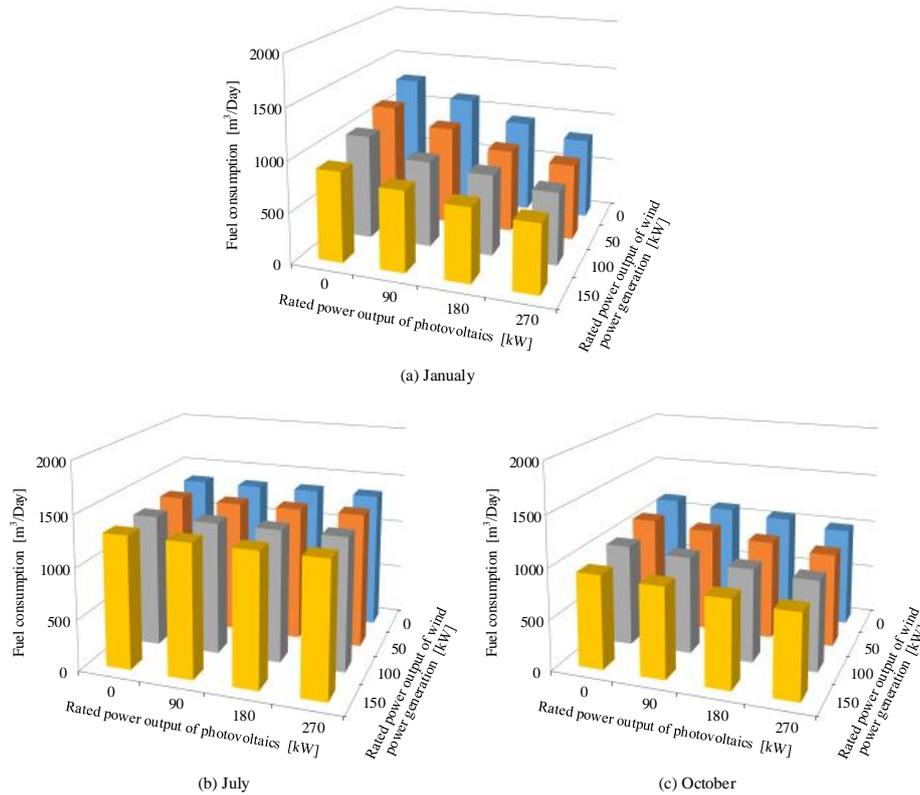
Fig. 20 Analysis results of the proposed system (System B). 5 % of heat supply to the heat pump.
