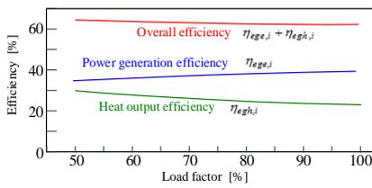
Fig. 13 Efficiency characteristics of the 113 kW engine generator installed in SBMG
