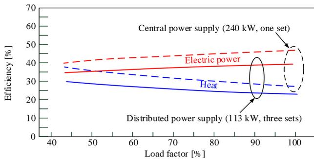
Fig. 5 Performance of the engine generator of a central and distributed system
