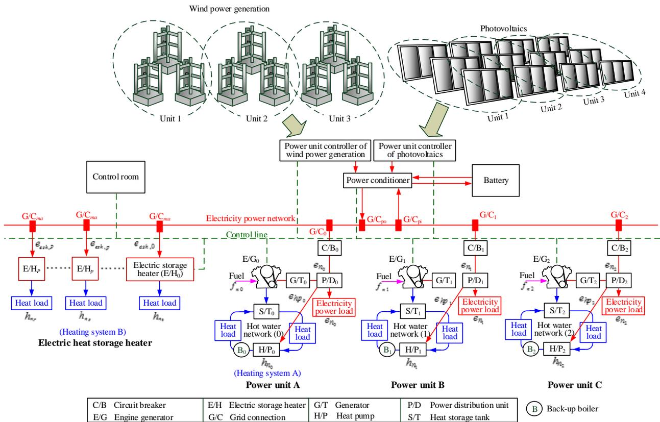
Fig. 2 Energy flow of the proposed microgrid
