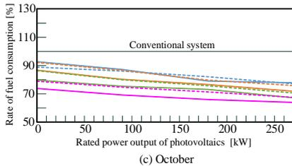
Fig. 14 Analysis results of fuel consumption rate of System B relative to the conventional system. Heat supply to all buildings except the power-generation (A\_0), residence (A\_1, A\_2), warehouse and sewage disposal (A\_3), administration (A\_4) buildings, which are shown in Fig. 1.
