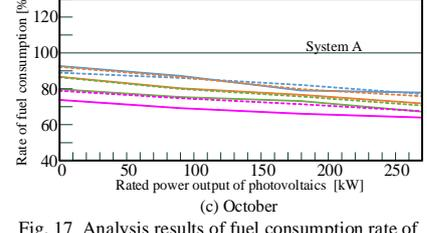
Fig. 17 Analysis results of fuel consumption rate of System B relative to the conventional system. Heat supply to the following buildings: power-generation (A\_0), residence (A\_1, A\_2), warehouse and sewage disposal (A\_3), and administration (A\_4) buildings, which are shown in Fig. 1.
