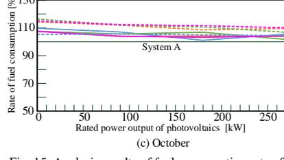
Fig. 15 Analysis results of fuel consumption rate of System B relative to System A. Heat supply to all buildings except the power-generation (A\_0), residence (A\_1, A\_2), warehouse and sewage disposal (A\_3), administration (A\_4) buildings, which are shown in Fig. 1.
