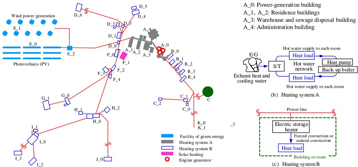
Fig. 1 Configuration of the electric power network and heating system of the Syowa Base
